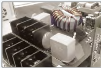
Built-in EMC Filter (C2 class)
